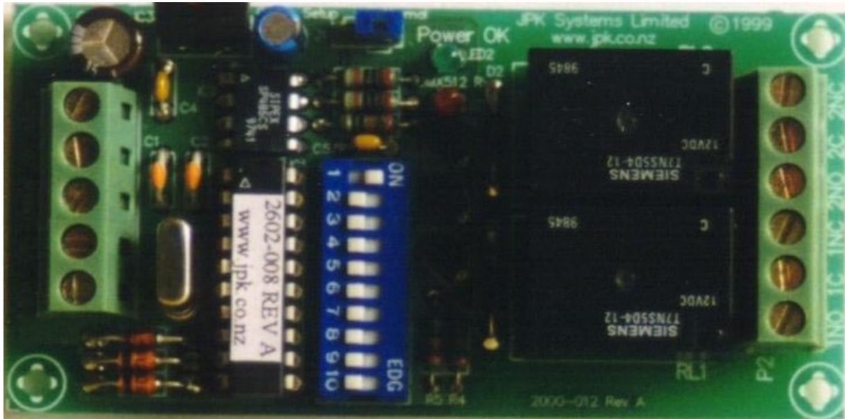
DMX contactor boards by JPK Systems Ltd provide both normally open and normally closed isolated contacts capable of switching low current signals and high current power loads. Integration of existing equipment into a DMX512 lighting control system is easy and cost effective.
